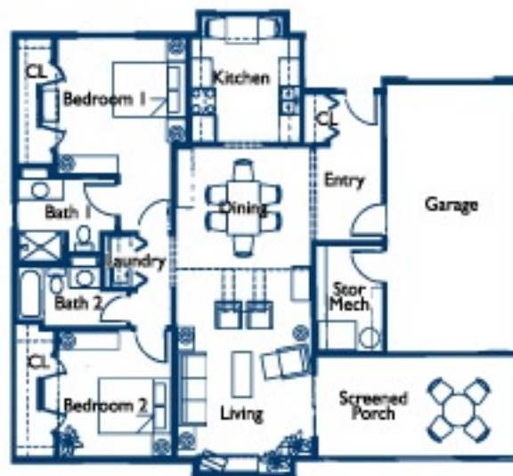
Cottage #2 1,958 Gross Sq. Ft. • Living Space: 1,421 Sq. Ft. Porch & Garage: 537 Sq. Ft.
